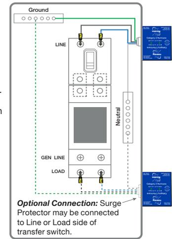
**Optional Connection:** Surge Protector may be connected to Line or Load side of transfer switch.
