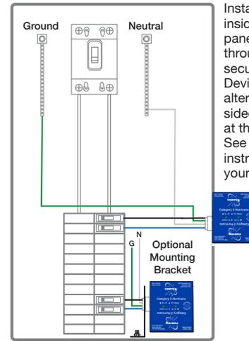
Install small L-bracket inside of the electrical panel. Insert nipple through L-bracket and secure with locknut. Device may be secured alternatively using double sided tape, when placed at the bottom of the panel. See diagram A for wiring instructions, depending on your application.
