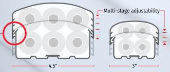
**Interior Adjustable Tabs** allow the cover to quickly snap in and secure the cover in place. (Multi-zone = 4 tabs; Single zone = 3 tabs)
